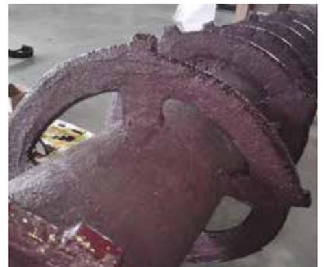
Screw Auger coated in Belzona 1811
