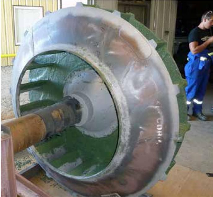
Belzona 1813 is a two-component repair and protective coating for surfaces subject to abrasive attack at elevated temperatures up to 200°C (392°F).
